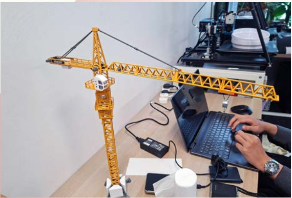
Plastic models are insensitive. Use metallic model instead
