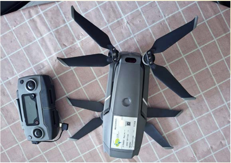
Drone to measure coordinates of a construction crane
